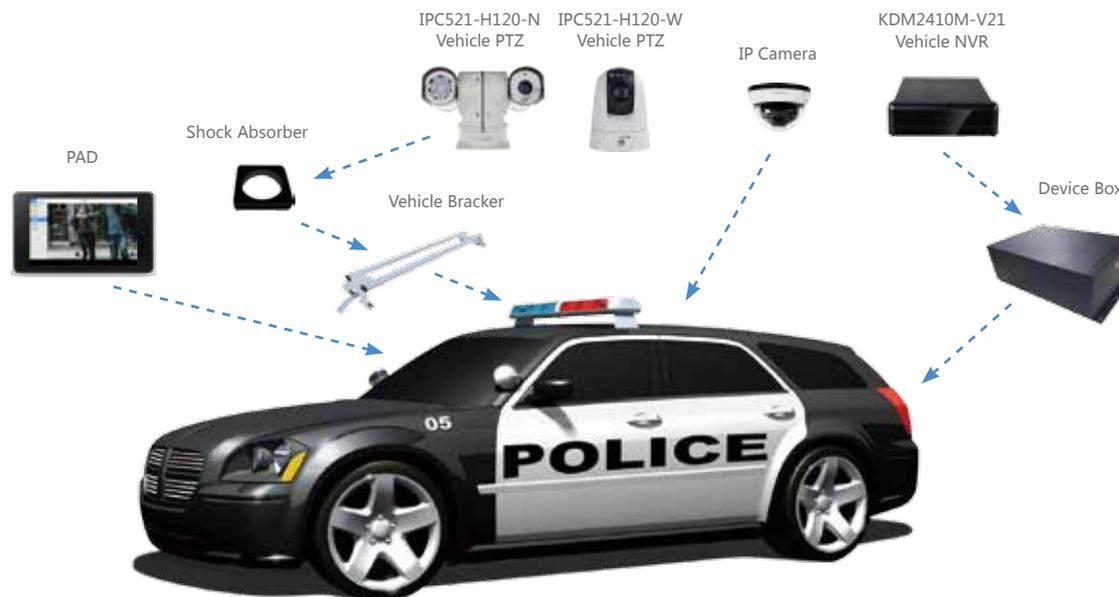
The embedded communication functions within the KVMS works through 3G/4G and wireless network while audiovisual data is uploaded to command center and shared with users within the same networking group. The KEDACOM KWTP wireless protocol used by our system ensures very low latency and drastically reduces packet loss for video streaming while delivering superior image quality.
