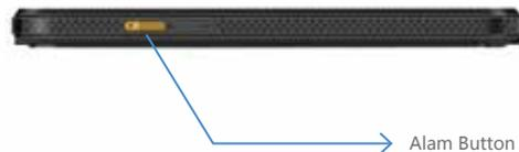
A pre-defined emergency button is created for the IPW200. In case of an emergency, by pressing this button the command center is alerted by means of an alarm to merit a swift centralized response.
