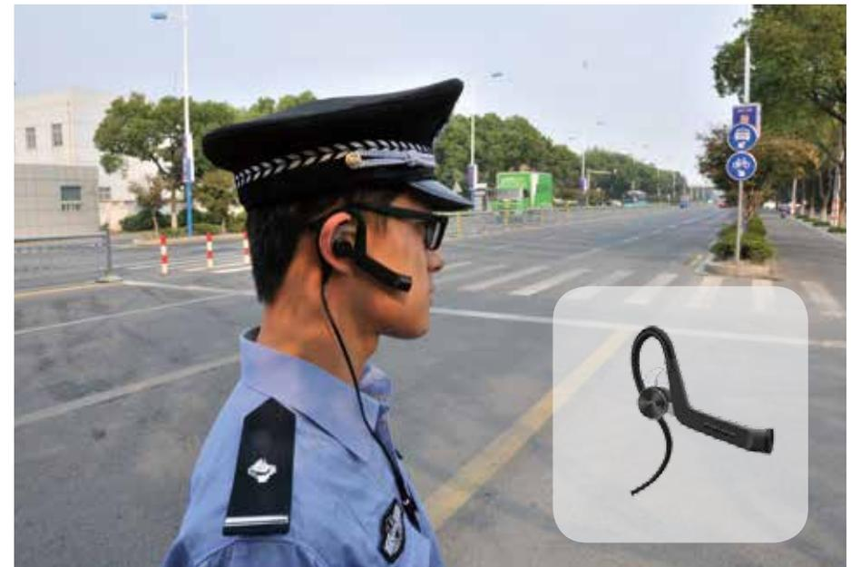
USBCAM-200 is an ear-hook camera which can be used together with IPW200 and DSJ-U1. On first glance, It looks like a Bluetooth headset from appearance but it enables true covert surveillance. USBCAM-200 also has a lens with F2.2 large aperture and diagonal Field of View (FOV) up to 100°, to acquire videos at 720p@30fps. The built-in microphone and headset can be used for communication with command center in intercom mode.
